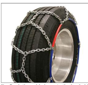
4) Push the cable hoop to the backside making sure the cross chain are centered on the tread face.
