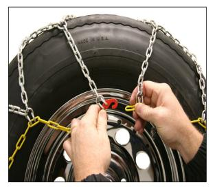
3) Pull side chain together to the center of the tire and hook the red flat fastener into one of the links.
