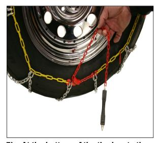
5) At the bottom of the tire locate the red fastener and red draw chain. Pull both outward to eliminate slack and tangles. Feed the red draw chain around the opening of the fastener and pull the draw chain tight, locking a link into the notch on the fastener.
