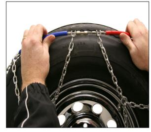
Grasp the two ends of the cable and pull outward and toward the top of the tire, then fasten tightener.
