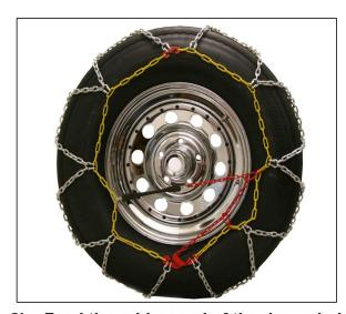
6) Feed the rubber end of the draw chain through the red rings. Stretch the rubber handle tight and hook on the adjacent side. NOTE: It may not be possible to use both red rings on some tire sizes. However, use both rings when possible. Move vehicle at least 15 feet and retighten chains.
