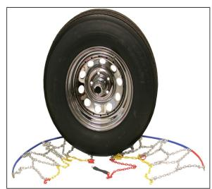
1) Lay the chain on the ground and remove any tangles. Make sure the hook ends are facing the ground. Starting with the red end of the cable, slide the cable and chain behind the tire.
