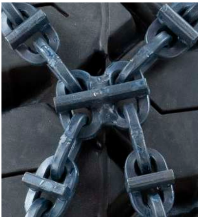
WEAR BAR CLOSE-UP
